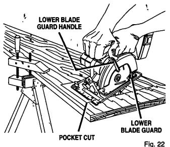
Depress the lock-off button and squeeze the switch trigger to start your saw. Always let the blade reach full speed then slowly lower blade into the workpiece until base is flat against workpiece.
